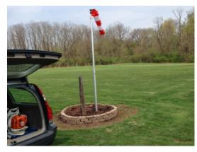
This year we added a new "airport" quality windsock to the field. It was set at a height that captures the wind velocity below the tree line at takeoff and final landing heights just above the runway. As many of you know, wind velocity changes can be significant above the tree line. Let us know, does this windsock meet your needs or do you prefer to know the wind velocity at a higher elevation than this?
